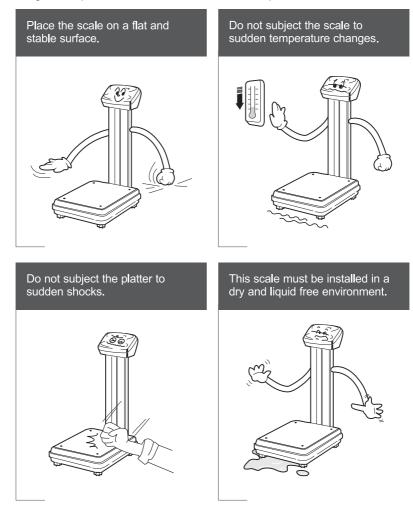
If the scale is not properly level, please adjust the 4 legs at the bottom of the scale (turn legs clockwise or counterclockwise) so as to center the bubble of the leveling gauge inside the indicated circle.
