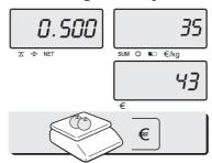
(1) Place an item on the platter and press  $\mathbf{\in}$  key in the normal weighing mode
