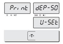
① Press **ZERO** key to move next function set selecting the printer.
