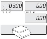
(5) After weighing item remove all of the container from the platter.
