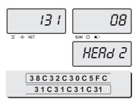
(4) Using ASCII code you can input appropriate data on Header 2. Ex) 820-1111, telephone #.
