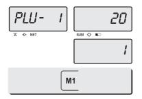
③ Press PLU key (M1 ~M4) to input a direct PLU address.
