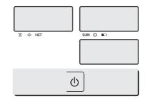
② Press the **ON/OFF** key for a few seconds to turn off.
