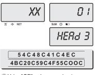
(6) Using ASCII code you can input appropriate data on Header 3. Ex) THANK YOU
