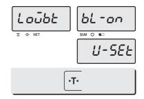
① Press **ZERO** key to move next function setting, low battery backlight auto off..
