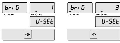
③ Press **ZERO** key to move next function setting, backlight brightness.
