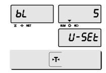
① Press **ZERO** key to move next function setting, backlight **ON/OFF.**
