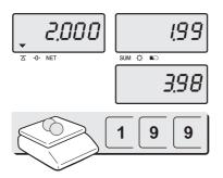
① Place an item on the platter and press appropriate numeric keys to input unit price. EX) 1.99 for unit price.
