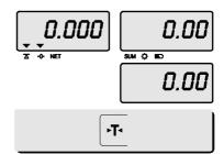
② Press **TARE** key to exit to normal weighing mode or **C** key up to maximum 8th byte. Then automatically exit to normal weighing mode.
