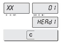
① Hold down C key and press ON/OFF key under the scale power off. "O1" on the "Unit Price" display represents that you are ready to input the first character.
