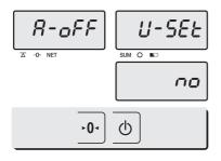
① To get into "User's Set-up Mode" press ON/OFF key pressing and holding ZERO key.
