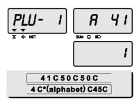
Input appropriate ASCII codes to save the PLU name.
