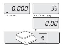
④ Remove the item from the platter. and press € key to go back to the normal weighing mode.
